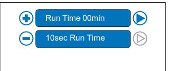
**Rinse Delay Time** – Configurable delay time for rinse, when the rinse signal is received to the RINSE INPUT the delay time will activate before allowing the rinse pump to operate
